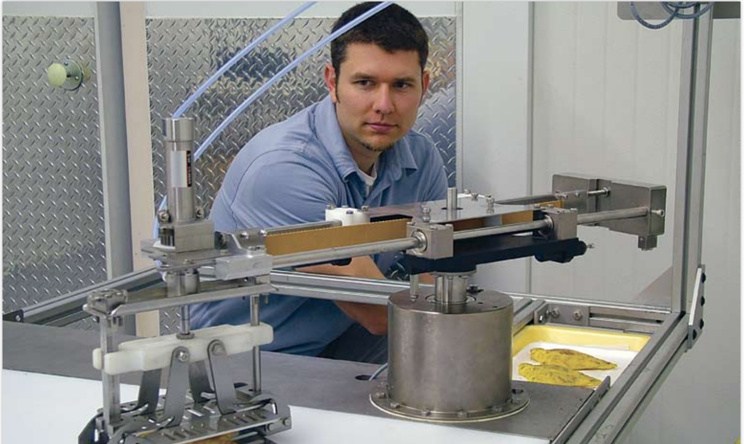
A GTRI researcher studies operation of components in a new “washable” robot designed for use in poultry processing.
