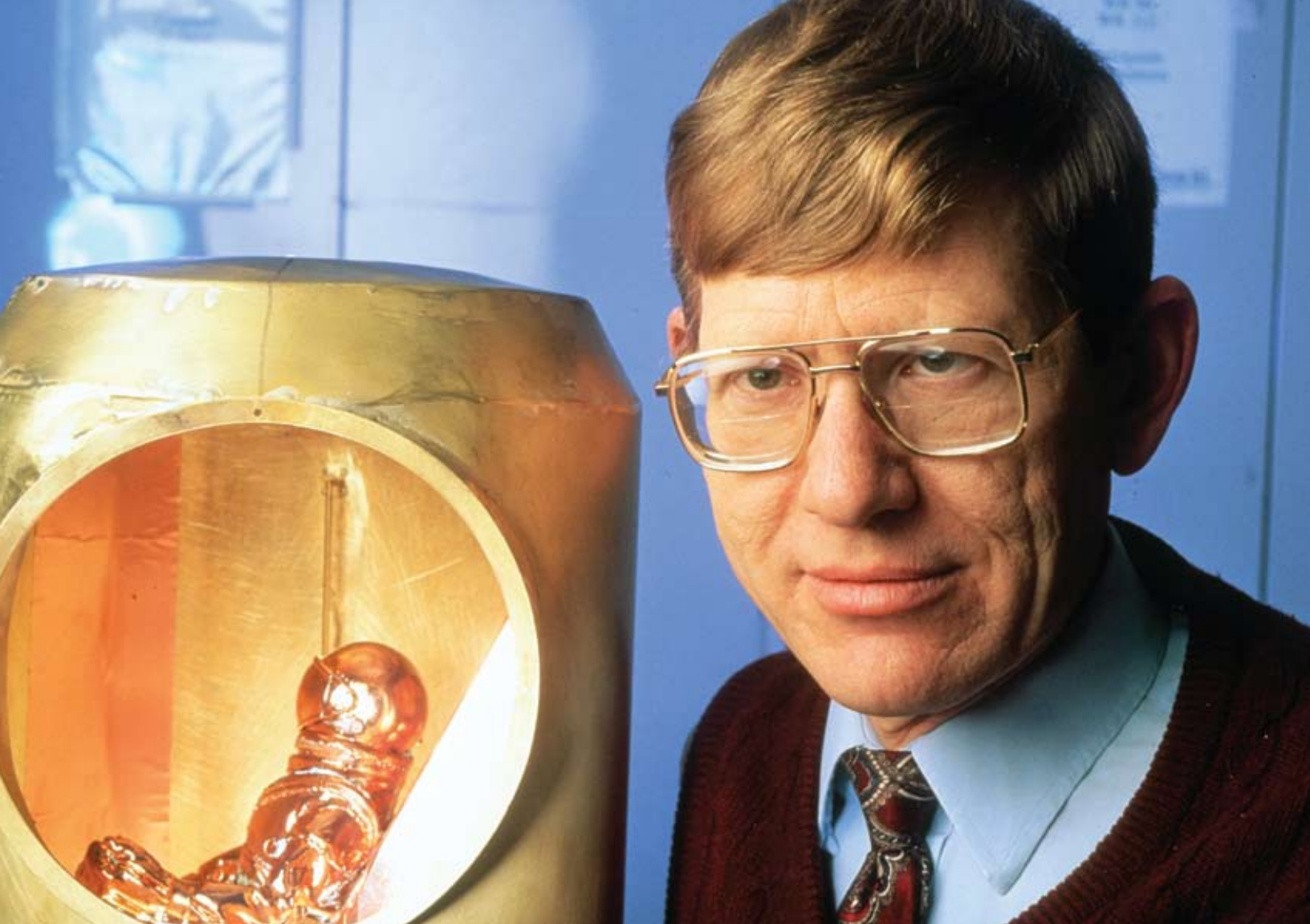
GTRI engineer Vic Tripp is shown with a scale model astronaut used to simulate operation of a “towel bar” antenna for use inside the air lock of the International Space Station.
