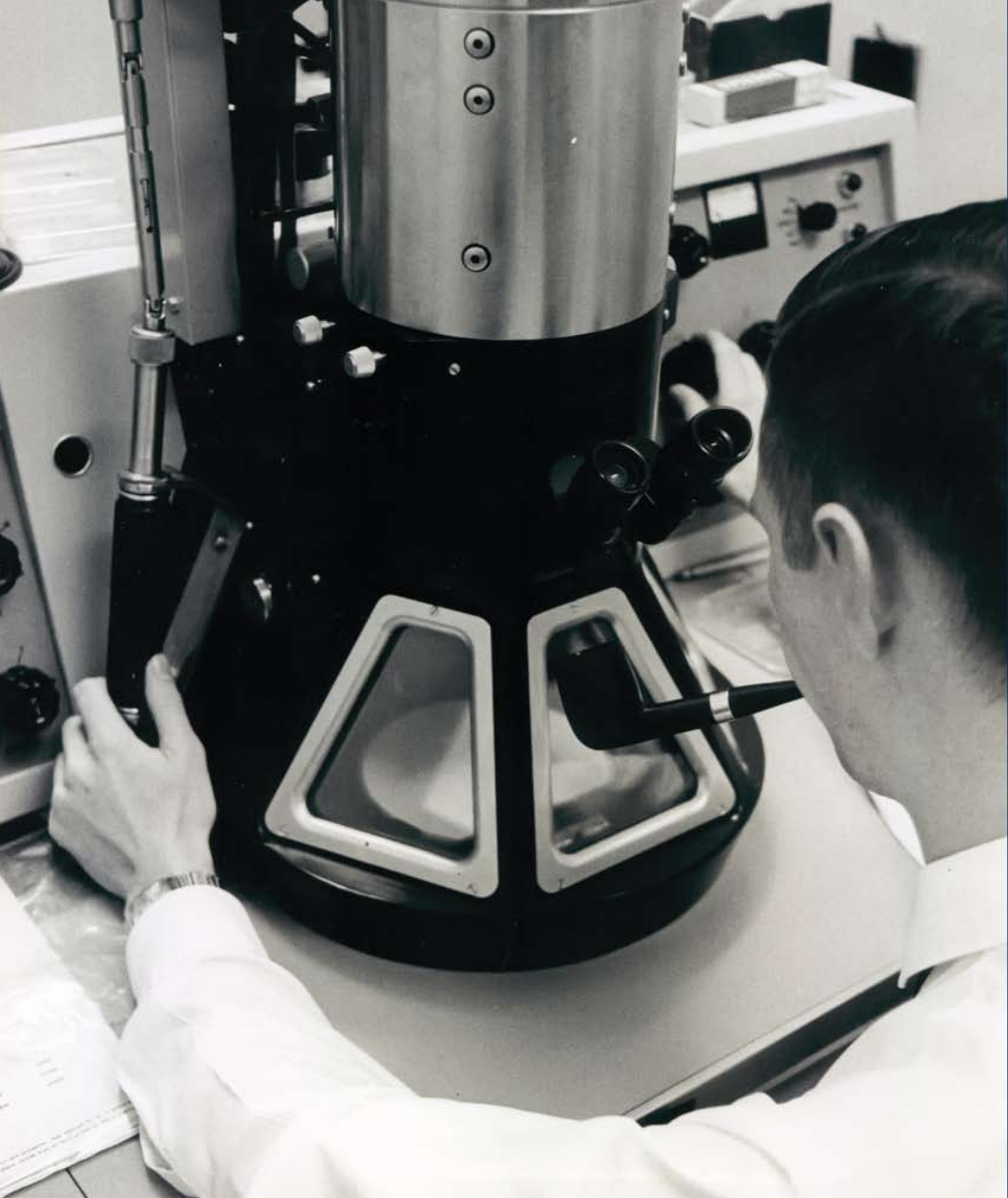
In 1947, the Engineering Experiment Station (EES) installed one of the first electron microscopes in the United States. The device was used for research on kaolin.
